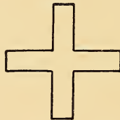
Fig. 86. Showing the shape of a machine drill bit before cutting bevel to form cutting edge.
